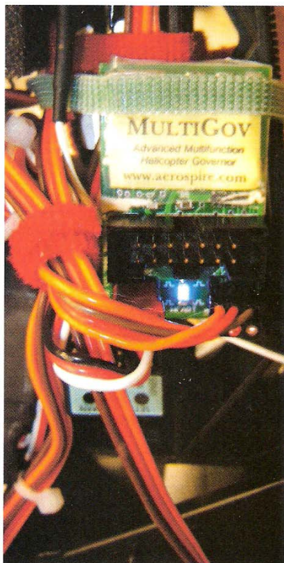
An onboard status light verifies an acceptable pre-start and post-start engine run condition. It can indicate a bad battery, questionable connections or a poor sensor signal. It also serves as an index reference for servo plug insertion
