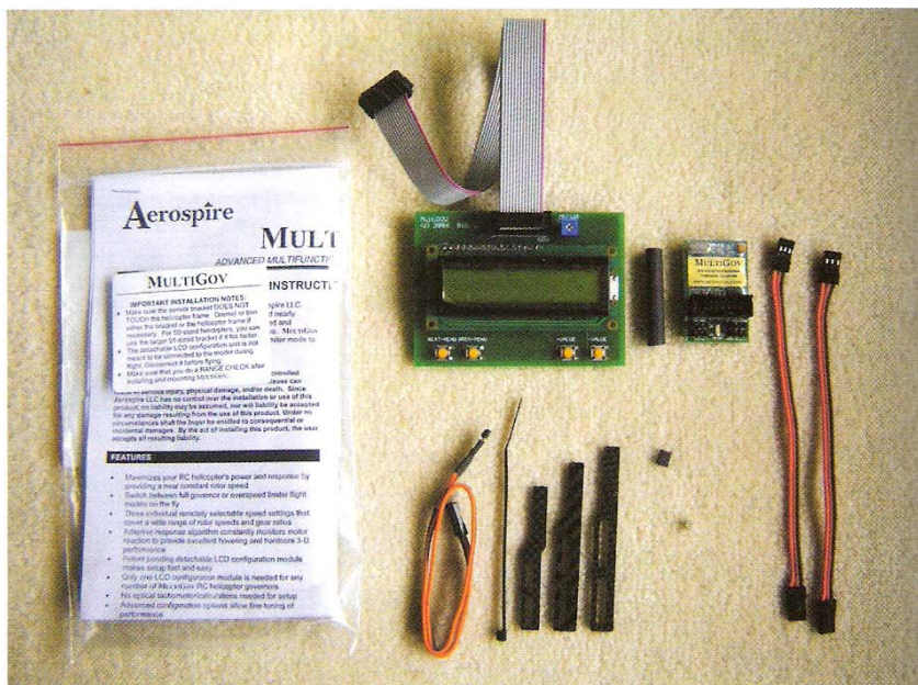
The MultiGov contains everything needed to install the unit to most 30-90 helicopters
