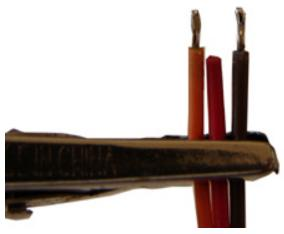
**Step 2:** Solder wires to thermistor chip and trim any excess wire protruding above the chip. A tweezer is being used to hold the chip for easy soldering.
