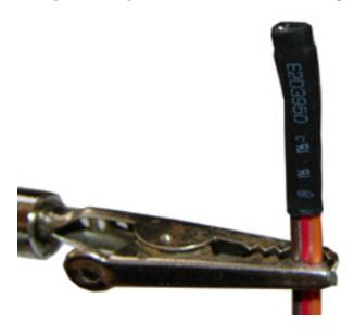
Construction is complete. Test sensor by plugging into "Tmp" of MultiGov Pro and going to the "Current" menu. If the sensor is working, the current room temperature will be shown on the LCD (the temperature should rise if you hold the sensor at the tip). If there is a problem, you will see "TEMP SEN NO CONN".
